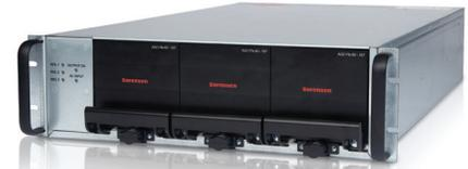
The ASD FLX with its 3U, 30kW water-cooled packaging provides one of the highest power densities available with outstanding output ripple and noise. The water-cooling allows for use in environments that normally exclude air-cooled power supplies.
