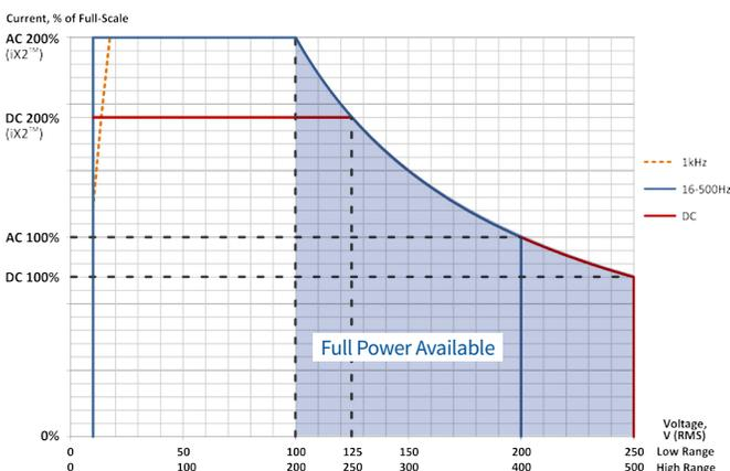
All Asterion sources employ AMETEK's latest current enhancing technology, iX2™. The iX2 current doubling technology enables output current to increase linearly up to two times the full output current as the voltage decreases from range maximum to one-half of range voltage. iX2 technology results in a source that delivers full power over the widest voltage ranges. This eliminates the need to buy overpowered sources just to reach low line current requirements.
